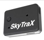
**Power On:** To power SkyTraX on, press and hold the button until the purple indicator LED turns off.
